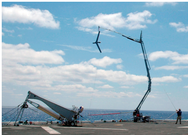
Figure 1. ScanEagle ® unmanned aerial vehicle (UAV) (Boeing Insitu, Bingen, WA, USA) lands on skyhook for recovery. The SuperWedge ® pneumatic launching catapult (left) can be mounted on vessels. © United States Navy.
